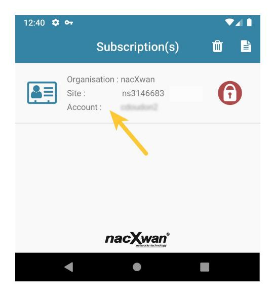
On clicking a subscription, the login interface appears. It takes certain information and indicates the status of the VPN, here for example it is disconnected (Red Padlock). It is also in this interface that it is possible to see the services that are secure
